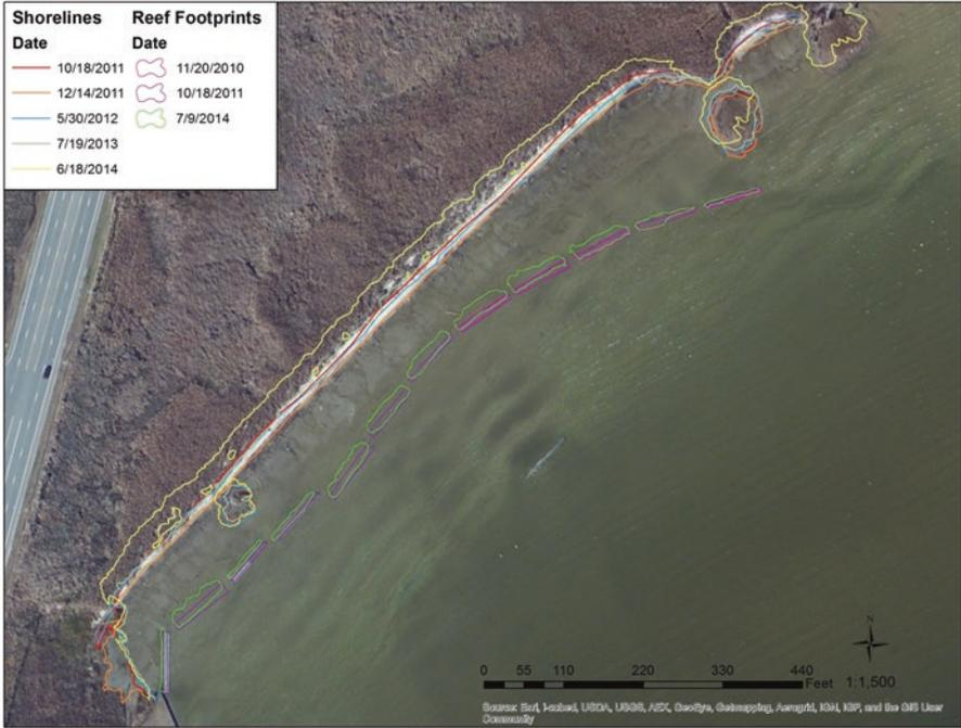
**Fig. 13.5** Reef footprints at Helen Wood Park with purple lines showing as built outline in spring 2011. The green line (2014) shows changes after 3 years. The reefs measured ~25 m long and 2–3 m wide with 7.5 m gaps. The two reefs on the left are bagged oyster shells and the reef on the right is made of Reefballs. The second reef on the right is partly made of Reefballs (right side) and partly bagged oyster shells (left side)
