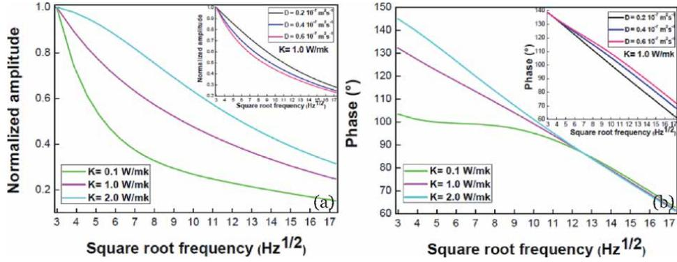
**Figure 5.** Theoretical variation of the normalized amplitude (a) and phase (b) of the photothermal signal with the square root of modulation frequency for three values of thermal diffusivity and thermal conductivity.
