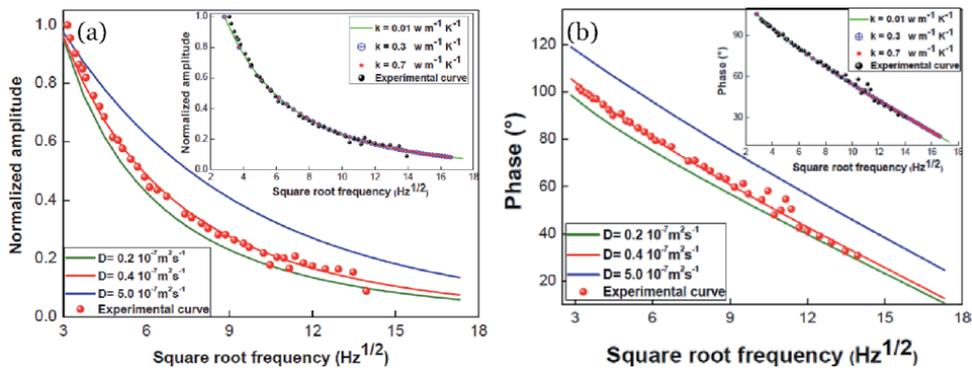
**Figure 6.** Experimental and theoretical variation of the normalized amplitude (a) and phase (b) of the photothermal signal with the square root of modulation frequency for three values of thermal diffusivity and thermal conductivity.
