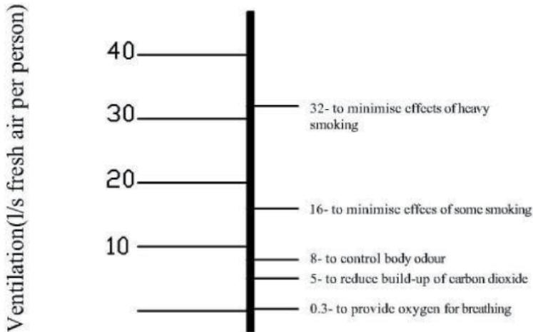
**Figure 1.** Ventilation rates for fresh air control [26].
