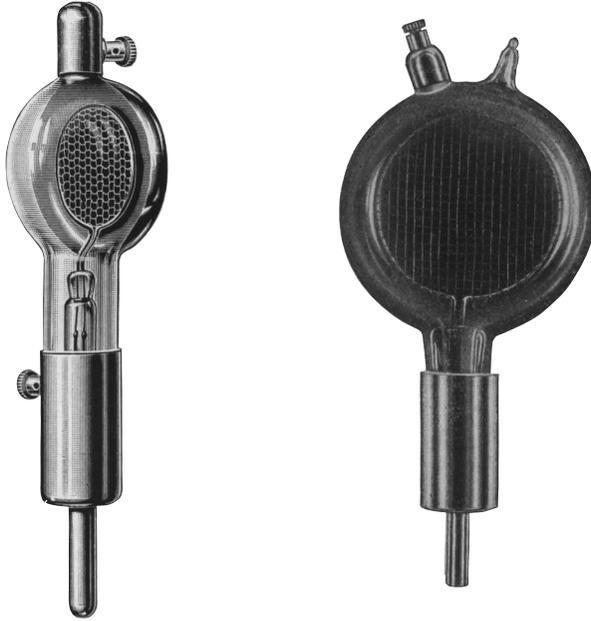
**FIGURE 14.** Photoelectric cells. These tiny devices transduce light into electricity; they were central to the development of optical sound film. Source: Heinrich Geffcken, Hans Richter, and Joachim Winkelmann, *Die lichtempfindliche Zelle als technisches Steuergerät* (Berlin: Deutsch-Literarisches Institut J. Schneider, 1933), 37.
