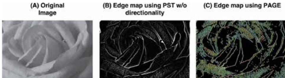
**Figure 6.** Comparison of feature detection using phase stretch transform (PST) and phase-stretch gradient-field extractor (PAGE) the original image is shown in (A). The output edge image obtained using PST without the support of directional response is shown in (B). The edge map obtained using PAGE filter banks that support edge detection at all frequencies is shown in (C). Different color values are used to show the orientation of the edges.
