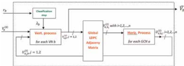
**Figure 14.** Block diagram of the overall classification-based decoder.
