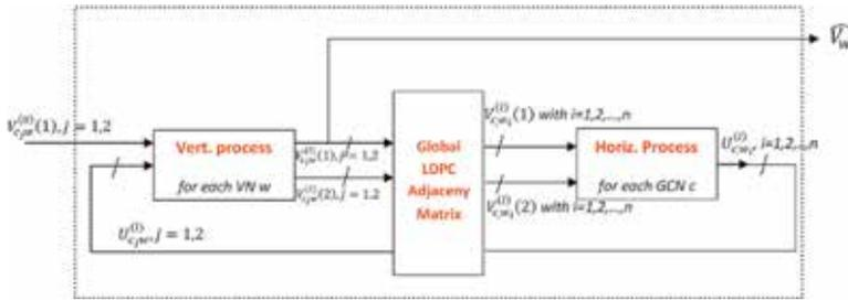
Figure 9. Block diagram of the overall TSSA-BF decoder.
