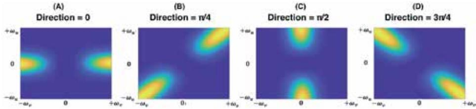
**Figure 4.** Phase-stretch gradient field extractor (PAGE) directional filter banks (A)–(D) the directional filter banks of PAGE computed using the definition in Eqs. (9)–(13) for steerable angle  $\theta = 0, \pi/4, \pi/2$  and  $3\pi/4$ , respectively. By monitoring the value of sigma  $\sigma_w$  of the normal filter  $\phi_1(u')$ , the angular spread of kernel  $K[u, v, \theta]$  can be controlled to avoid any overlapping of directional filters.
