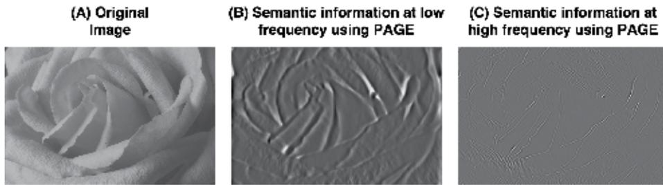
**Figure 7.** Feature detection using phase-stretch gradient field extractor (PAGE) at low and high frequency: Features detected at low frequency are much smoother whereas for high frequency, the features are sharper. This demonstrates the frequency selectivity for feature detection using PAGE.
