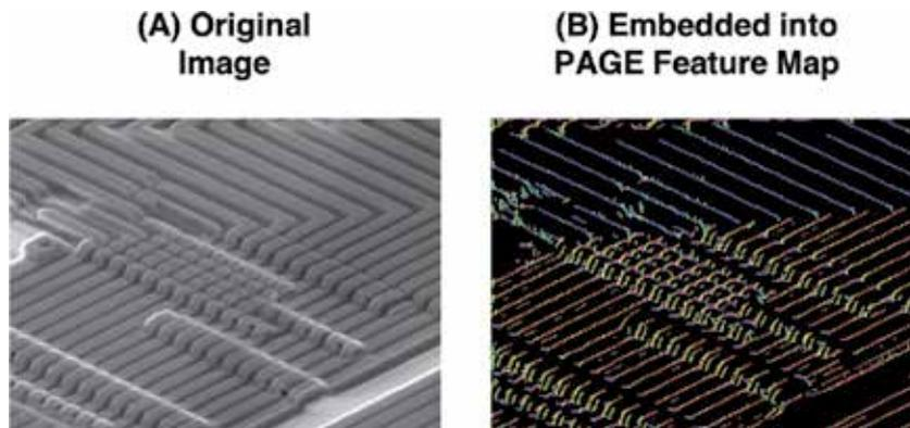
**Figure 10.** Fabrication artifact detection using phase-stretch gradient-field extractor (PAGE) on a single Electron microscope (SEM) image of integrated circuit chip. The original image is shown in (A). The output edge image obtained using PAGE filter banks that support edge detection at all frequencies is shown in (B). Different color values are used to show the orientation of the edges that correspond to the chip layout and can be used to detect fabrication artifacts.
