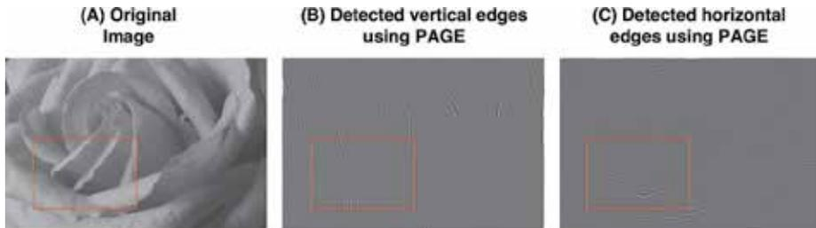
**Figure 5.** Phase-stretch gradient-field extractor (PAGE) directional filter banks response the original image is shown in (A). We design two directional PAGE filters here to detect vertical ( $\theta = \pi/2$ ) and horizontal ( $\theta = 0$ ) edges as shown in (B) and (C) respectively.
