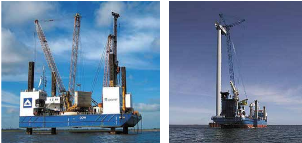
Fig. 5. Examples of external cranes for replacement of large components; Jack-up barge ODIN (left) and crane ship
