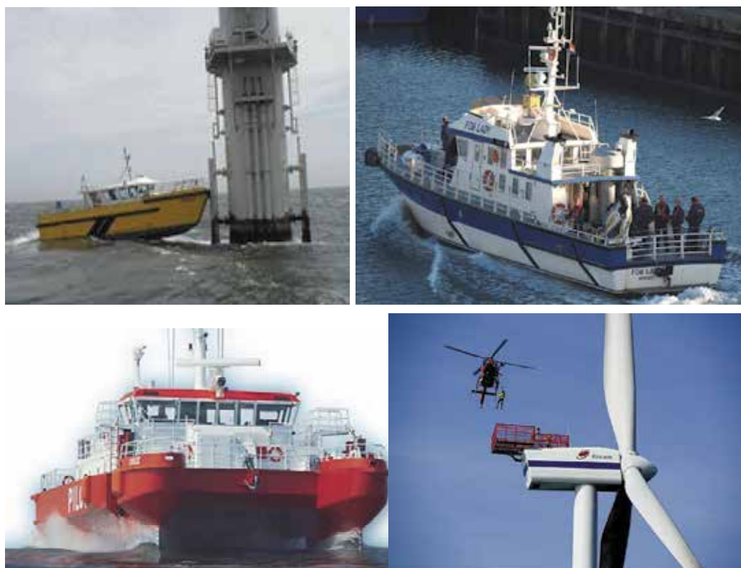
Fig. 4. Examples of transportation and access equipment for maintenance technicians; clockwise: Windcat workboat, Fob Lady, helicopter, and SWATH boat
