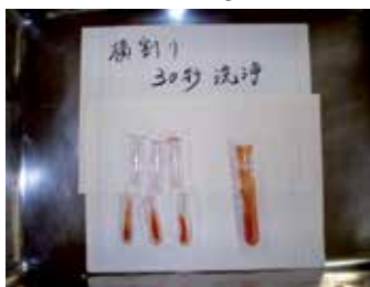
(c) Half length cut tubes after 30 second washing
