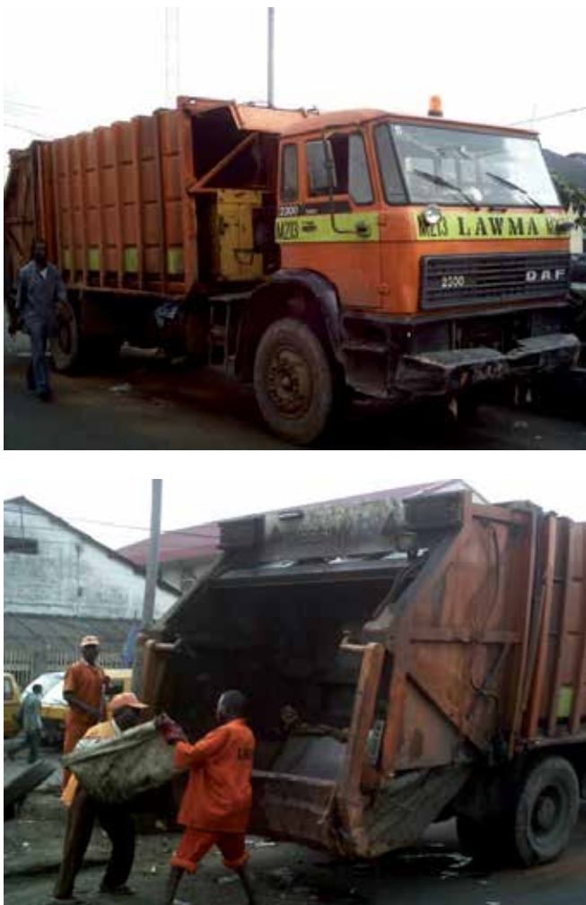
Fig. 1. Solid waste collection vehicles with hydraulic ram
