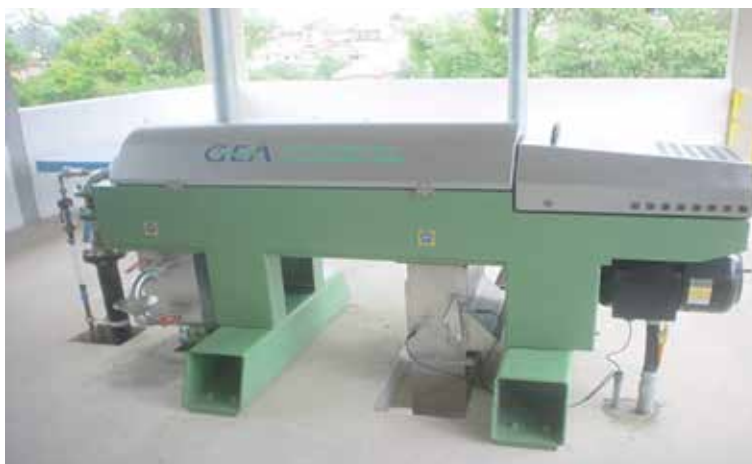
Figure 8. Photograph of a centrifugal decanter. WWTP-Sabesp, São Paulo, Brazil (source: the author).
