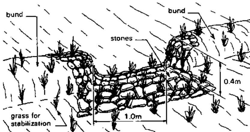
**Figure 32.** Spillway construction for bunds with external catchments (Pacey and Cullis, 1991).
