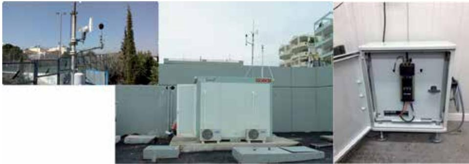
**Figure 1.** Permanent noise and air pollution monitoring systems deployed on Attiki Odos Ring Road, Athens, in use from 2001 to 2002: view of typical measurement stations and the CUBE measurement system (Dynacoustics & o1dB-ACOEM).
