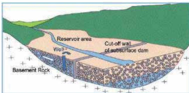
Conceptual Diagram of the Subsurface dam
