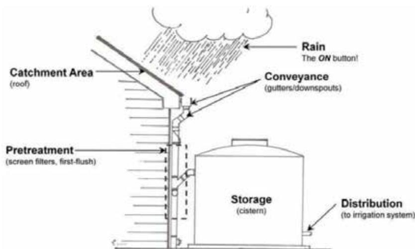
**Figure 1.** Components of a rainwater harvesting system (source: <https://slideplayer.com/slide/9100121/>).
