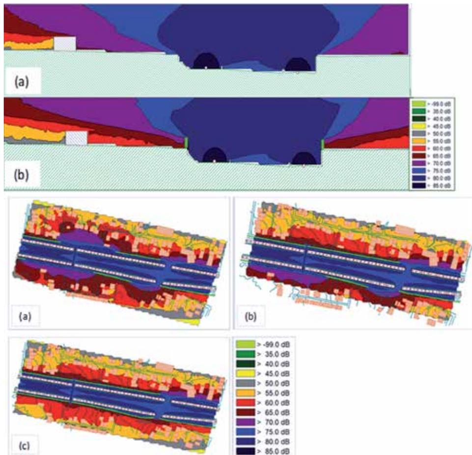
**Figure 8.** Athens Ring Road NAP (2017) [11]. Vertical grid—noise index  $L_{den}$ : (a) condition with no mitigation measures, (b) condition with the mounting of noise barrier. Horizontal grid—noise index  $L_{den}$ : (a) first scenario with no mitigation measures, (b) second scenario with barriers in two receptors, and (c) third scenario with barriers in three receptors (fully covered area).
