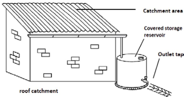
**Figure 2.** Rooftop catchment system (source: CTCN site).
