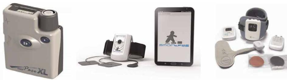
**Figure 7.** Functional electrical stimulation systems commercially available. From left to right: ODFS pace, SmartFES, and XFT-2001. Images obtained from the official website of SmartFES [68], XFT-2001 [69], and Odstock [70].
