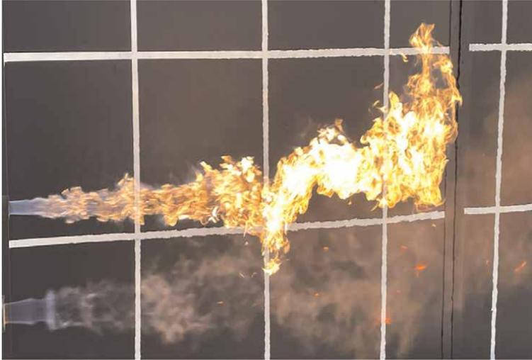
**Figure 3.** Natural gas (upper) and hydrogen (lower) oxyfuel flames with the same burner power.
