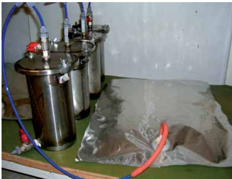
Fig. 2. Set of dry batch anaerobic reactors
