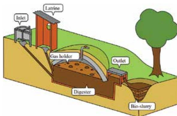
**Figure 3.** Schematic of biogas plant [12].
