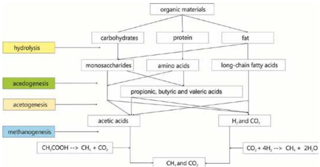
**Figure 1.** Conversion pathways of biogas production from biomass [10].
