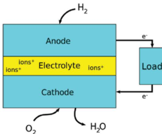
**Figure 4.** A block diagram of a fuel cell [13].
