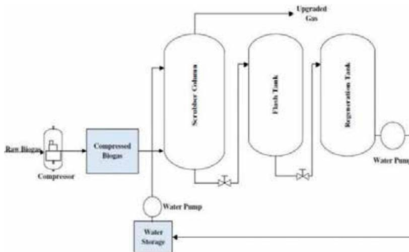
**Figure 5.** Schematic of chemical scrubber [28].
