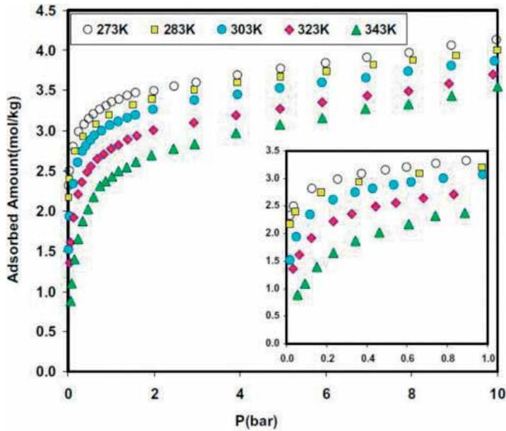
Figure 7. Carbon dioxide adsorption by zeolite [33].
