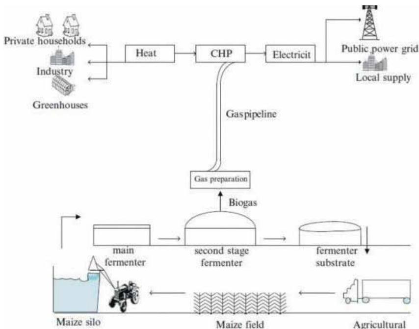
**Figure 3.** A typical maize-based biogas plant in Germany [20].
