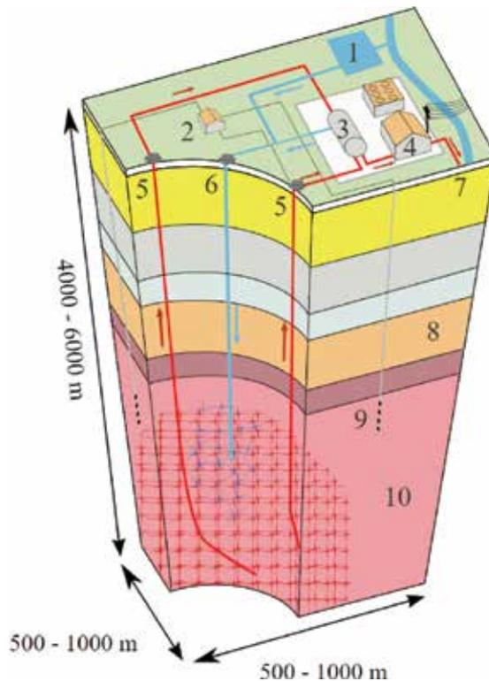
**Figure 2.** Geothermal system [12]. (1: reservoir, 2: pump house, 3: heat exchanger, 4: turbine hall, 5: production well, 6: injection well, 7: hot water to district heating, 8: porous sediments, 9: observation well, 10: crystalline bedrock).
