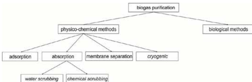
**Figure 4.** Biogas purification methods [27].
