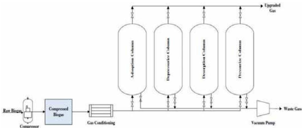
**Figure 6.** Schematic of adsorption in biogas purification [28].
