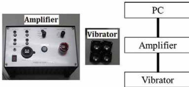
**Figure 8.** Photograph and block diagram of variable-frequency vibratory stimulation device.
