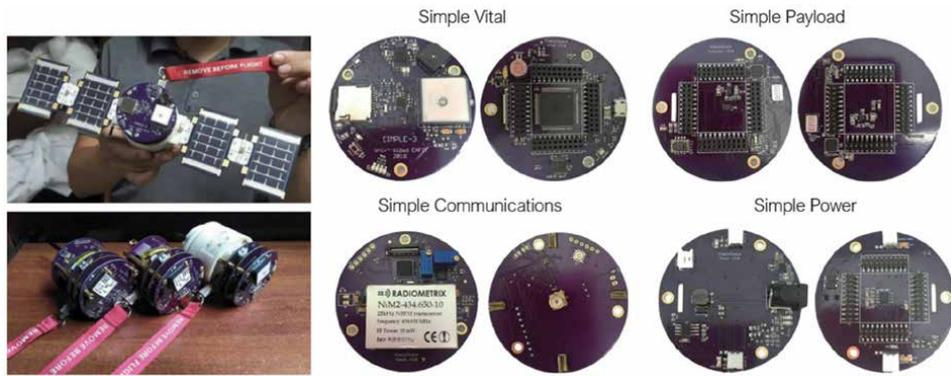
**Figure 7.** Low-cost sensing solution from SimpleSpace. The simple unit is divided in subsystems which can be adapted into a vertical bus which allows the insertion of new pcb layers with new measurement instruments.
