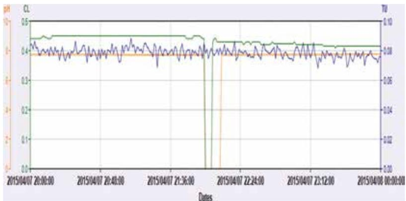
Figure 7. Malfunctioning of sensors.
