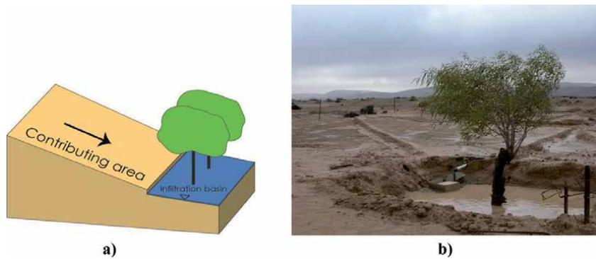
**Figure 6.** Traditionally designed micro-catchment system: (a) schematic of the system and (b) flooded micro-catchment.
