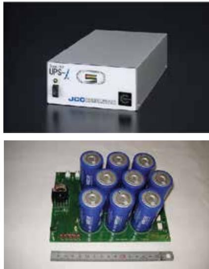
**Figure 1.** EDLC-based uninterruptible power supplies (UPSs).
