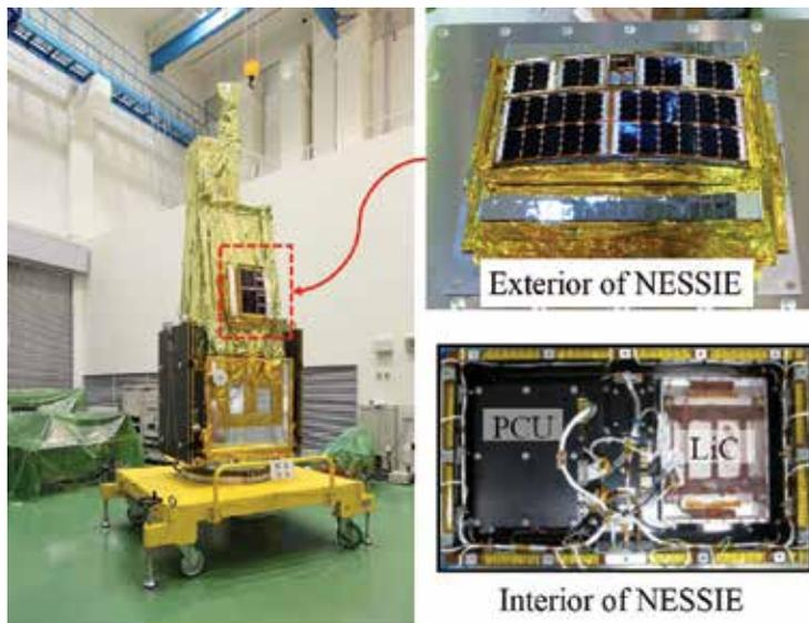
**Figure 16.** Photographs of NESSIE installed in HISAKI.
