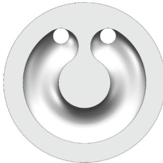
**Fig. 1.** Stator of vortex blower.
