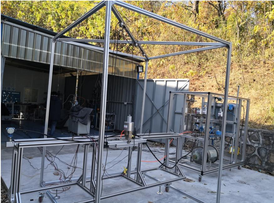
Fig. 2. High pressure hydrogen leakage and diffusion test facility
