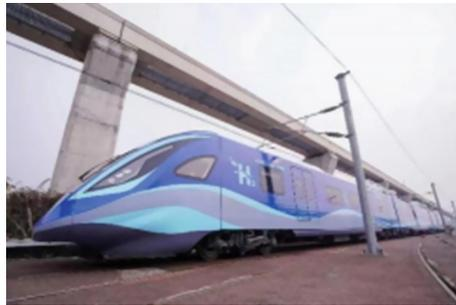
**Fig. 4.** The world's first hydrogen-powered regional express vehicle
