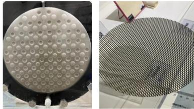
**Fig. 2.** Two common configurations of alkaline water electrolyzer: left, concave-convex bipolar plate (CCBP), right: metal 3D metal mesh.
