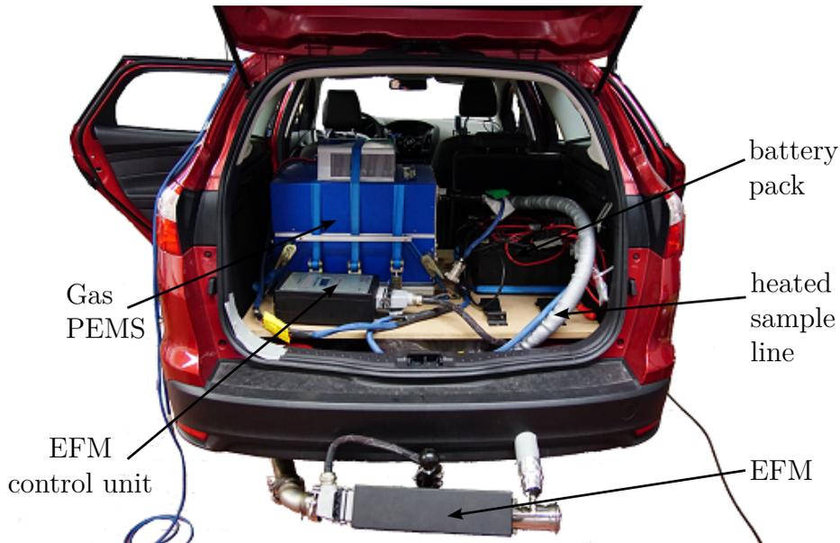
Figure 2.2: An example PEMS set-up showing the gas PEMS with accessories.
